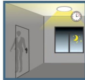
After the hold time, the sensor dims the lamp at the preset low light level if no motion is detected.
